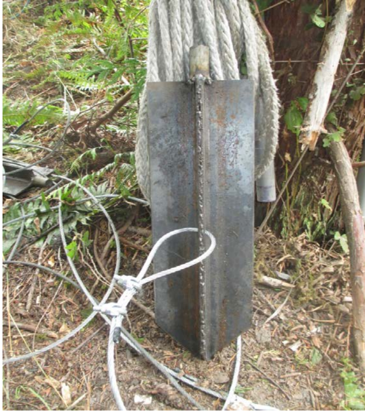
Figure 4. Redesigned “snow” anchor used to secure weir components in loose sediment.
